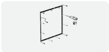
Let the current cable coming from the 24 VDC remote driver pass trough holeand position the pre-drilled metal clips supplied.
