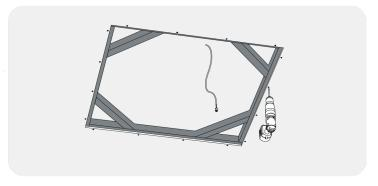
**2** Mount a reinforcement structure to the existing structure in order to fix the new plasterboard (plasterboard supplied).
