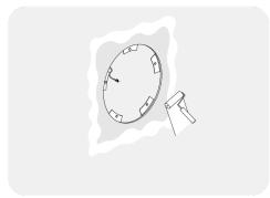
Connect the power cable, put the panel at the right position and turn it clockwise checking that the panel is well fixed before of leaving it.
