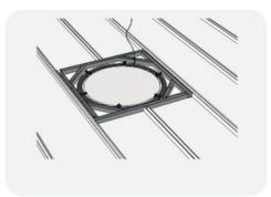
Put the adhesive mesh (not supplied) around the seam and plaster.
