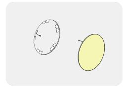
Put the adhesive mesh (not supplied) around the seam and plaster.
