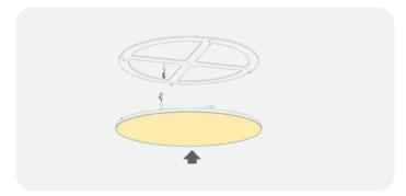
Dress the magnetic finish belt plate around the thickness of panel. If the belt seems too short, adjust the light circle position moving it a little bit; there is tolerance for this operation.
