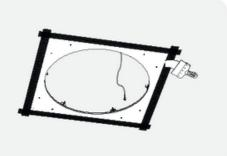
Connect the power cable, li§ the panel at the right position and turn it clockwise checking that the panel is well fixed before of leaving it.
