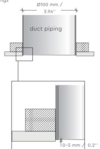
Make sure the ventilation ducts is positioned correctly. Then mount the Storm Plaster Ring according to the installation guide.
