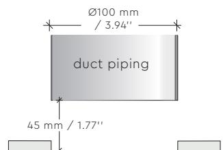
Make sure the ventilation duct is positioned correctly. Then mount the Back-Mounted Ring and Back-Mounted Adaptor according to their installation guides.
